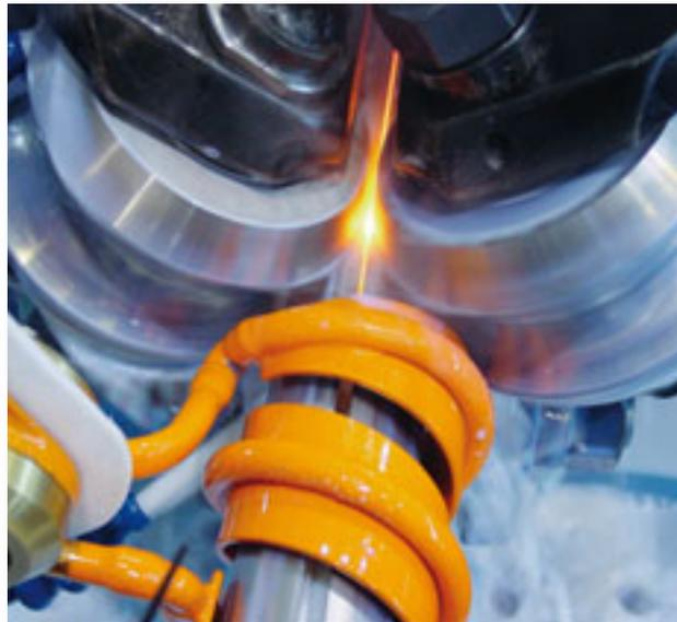
Welding head for 76 mm diameter tube
