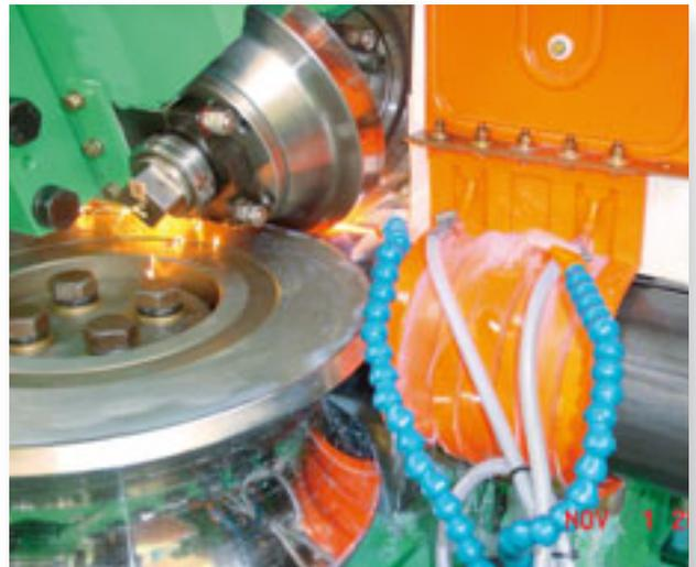
Weld area (160mm diameter pipe)
