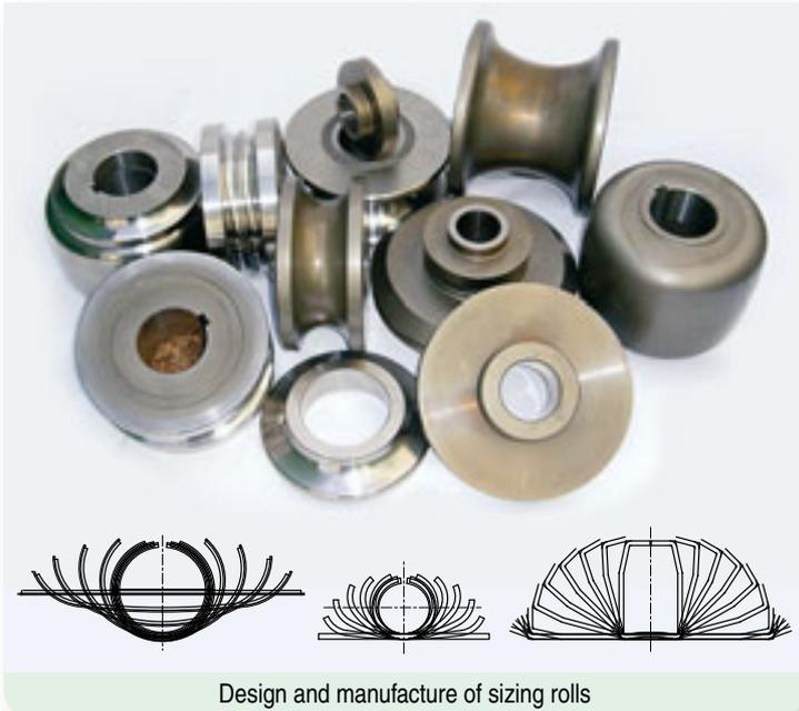
Design and manufacture of sizing rolls
